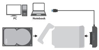
insert the HDD/SSD and connect to PC
